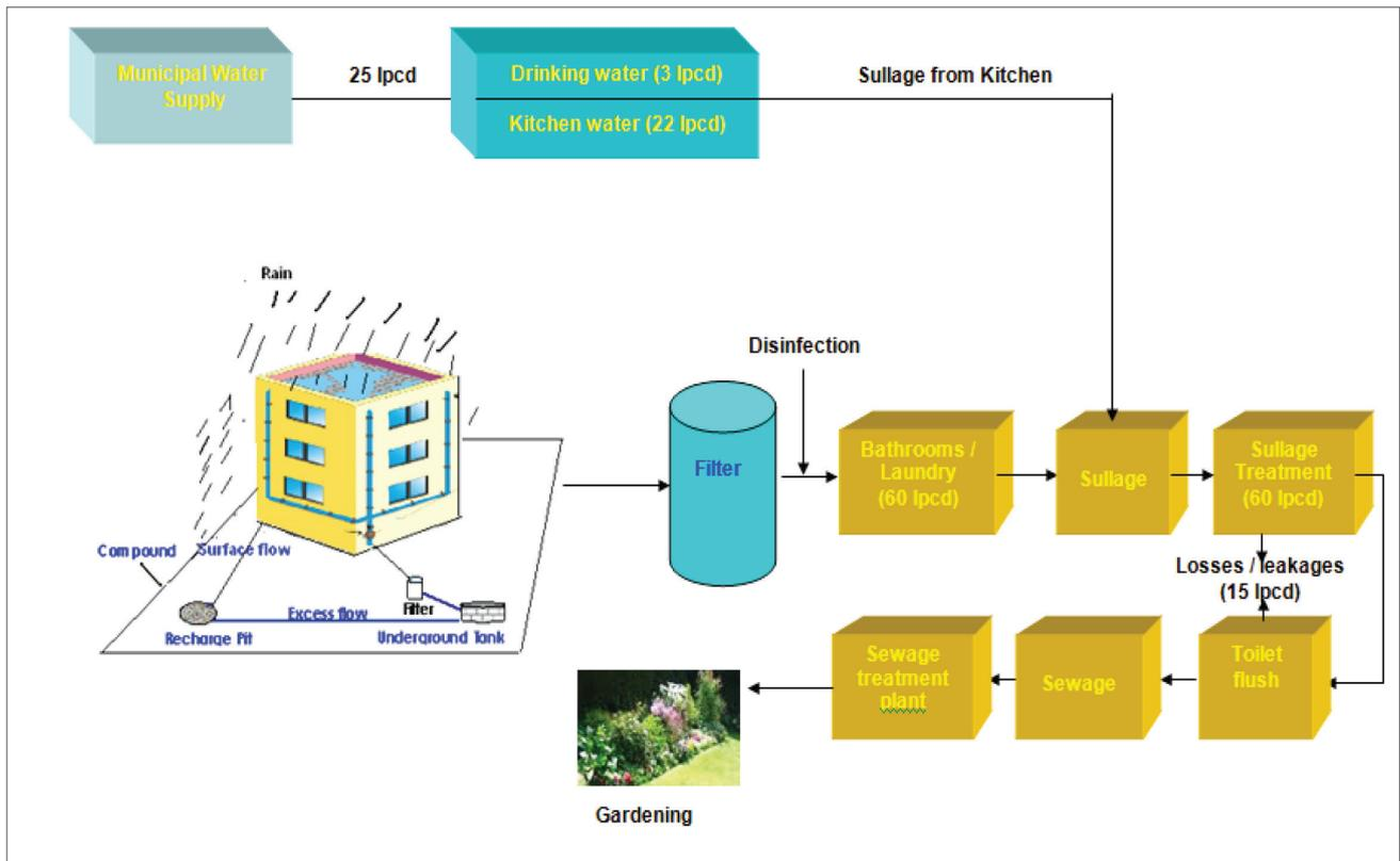
Figure 1: Total Water Management In Residential Complexes Using Rain Water And Sullage
