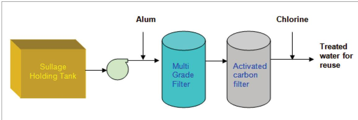
Figure 2: Sullage Recycle System
