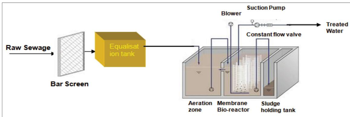
Figure 3: Treatment of Sewage Using Membrane Bio-reactor
